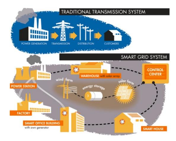
DER: Distributed Energy Resources include Distributed renewable generation sources, energy efficiency, energy storage, electrical vehicles, demand response technologies and utility grid modernization (e.g. Volt/VAR optimization (VVO), distribution automation)
